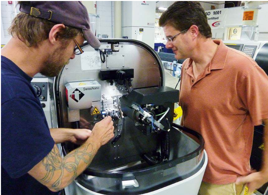
Petron's CNC Manager and Plant Manager fixing a 7-degree angle block in one of the new SwissNanos to manufacture a custom part for the Medical and Electronics industries.
