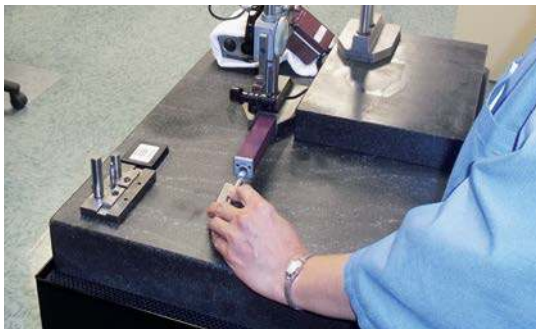
Quality Control engineers using a Profilometer to check ID finish for a part made in one of the EvoDeco 32.
