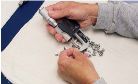
Quality Control engineers using a digital micrometer to check tight tolerances for a part made in one of the SwissNanos.
