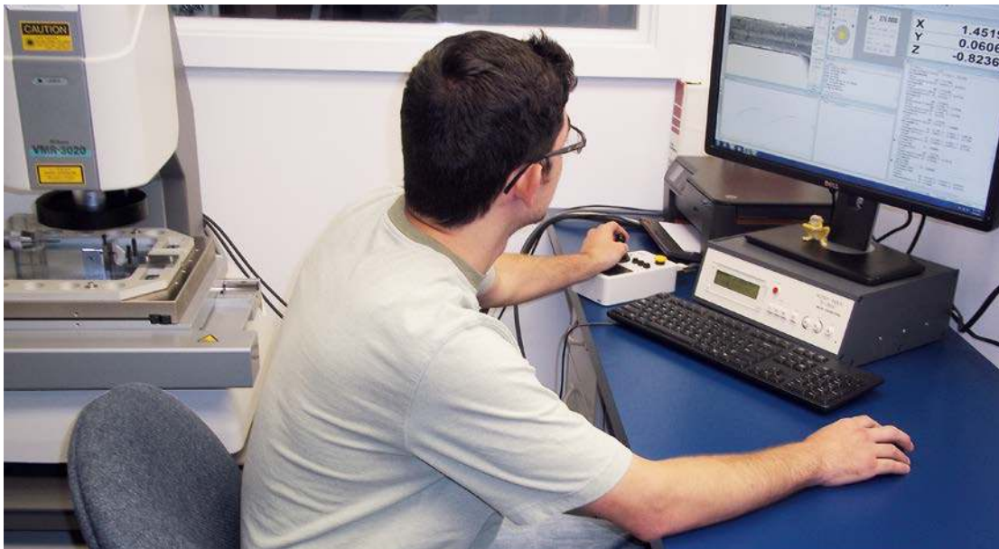
One of Petron's 4 Quality Control engineers using a Laser Vision System to check a part's dimensions from a part made in the EvoDeco 32.
